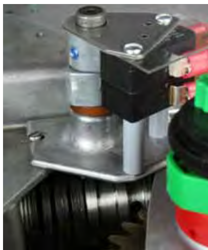
Torque Limit Switches shown with mounting bracket sectioned for clarity.
