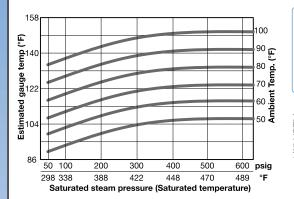
By knowing the saturated steam conditions and ambient temperature, the chart can estimate the gauge temperature, when the ABAC 's CV is used
