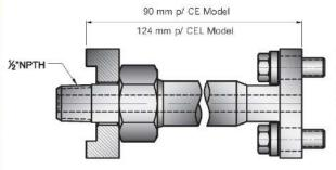
It is also available with a KD dielectric kit: dielectric isolation joint to avoid undesirable currents reaching the instrument and damaging it.
