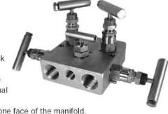
**Natural gas application:** The **M6GN** version has 3/8" orifice and soft seat. In this way it is possible to have bigger channels without diameter changes, to reduce pulsations in a gas line which may cause an error in the flow measurement as well as to assure a good drain where the wet gas and the hydrates are a problem.
